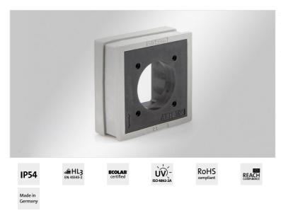
The grommet QT-AT-FL is constructed on the basis of a large QT cable grommet. The polyamide body is moulded with elastomer. All square flanges with dimensions 19.8 x 19.8 mm (M23) can be integrated.
